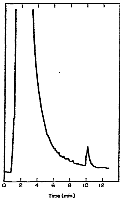
Fig. 6. Fluorescence-HPLC chromatogram for 5-ml cattle plasma sample containing 1.4 ng/ml dihydro-avermectin- B_{1a} .
